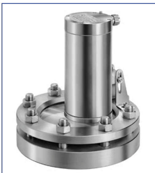
Sightglass light fitting type EdelEx 50 dH Sch K2, 50 W, 230 V, EEx d IIC T4, Ex II 2 G + D, mounted on circular sightglass to DIN 28120, PN 10, DN 150.
