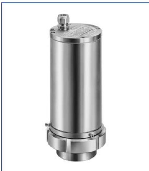
Sightglass light fitting type EdelEx G20 dH R 80 K1, 20 W, 230 V, EEx d IIC T5, Ex II 2 G + D, with intermediate flange collar fixation "R 80" mounted on a screwed sightglass similar to DIN 11851, PN 6, DN 80.
